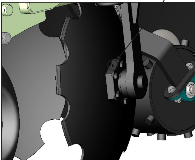
SIDE WALL BUSTER DISC BEARING (GREASE BOTH SIDES)
